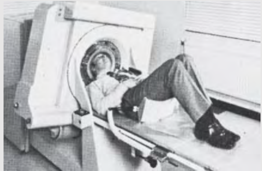
Figure 1-2 First-generation model of a CT head scanner. (Courtesy Thorn EMI, London, United Kingdom.)
